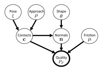
Fig. 3: A graphical model of the relationship between the uncertain parameters we consider. Uncertainty in object shape  $\theta$ , object pose  $\xi$ , and grasp approach angle  $\rho$  affect the points of contact  $\mathbf{c}$  with the object and the surface normals  $\mathbf{n}$  at the contacts. Uncertainty in friction  $\mu$  coefficient affects the forces and torques used to compute our quality measure, the probability of force closure  $P_F$ .
