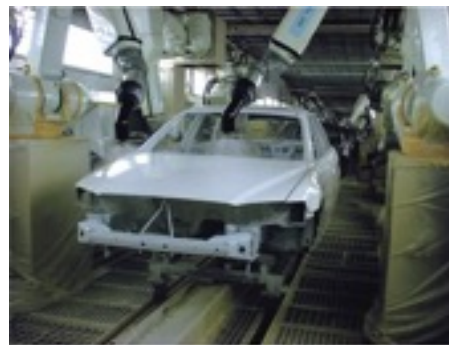
Automotive body paint line. (Courtesy of Kawasaki Robotics (USA) Inc.)
