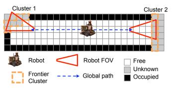
Fig. 5: **Global Planning**: We generate global plans by 1) clustering frontier voxels and 2) planning paths to destinations that can view them. When a robot can view a cluster from multiple places, we select the one that can be reached the fastest.
