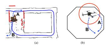
Fig. 10: **Limitations.** In (a) and (b) executing action A is preferable over action B as the robot's uncertainty will be much lower. However, our approach only considers the map's uncertainty and selects action B in both cases.
