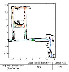
(a) Final map (2D projection), exploration path, and poses where trajectory optimization performed best: The green triangle is the robot's start position. The colored path is its exploration path. The red arrows show the 25 poses where trajectory optimization provided the largest gain in information over the initializing trajectory.
