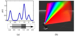
Fig. 3: Beam based measurement model: (a) one beam, the cells it intersects at various distances, and the resulting distribution over measurements when  $z_{\min} = 0.5$  and  $z_{\max} = 2$ . Darker cells have a higher probability of being occupied. (b) Raycasts for multiple beams. Obtained from Charrow et al. [5].
