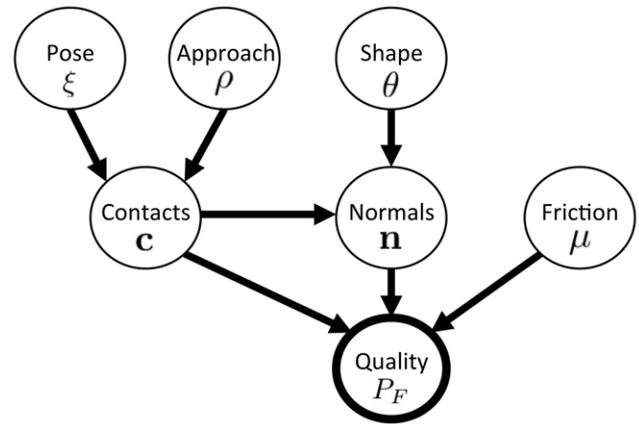
Fig. 3: A graphical model of the relationship between the uncertain parameters we consider. Uncertainty in object shape  $\theta$ , object pose  $\xi$ , and grasp approach angle  $\rho$  affect the points of contact  $\mathbf{c}$  with the object and the surface normals  $\mathbf{n}$  at the contacts. Uncertainty in friction  $\mu$  coefficient affects the forces and torques used to compute our quality measure, the probability of force closure  $P_F$ .
