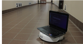
Fig. 1. A picture of robot (iRobot Create) in the operating environment. Landmarks can be seen on the walls.
