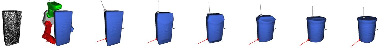
Example grasp transfer via a joint object/grasp deformation and optimization in  $\mathcal{G}^{rad}$ .
