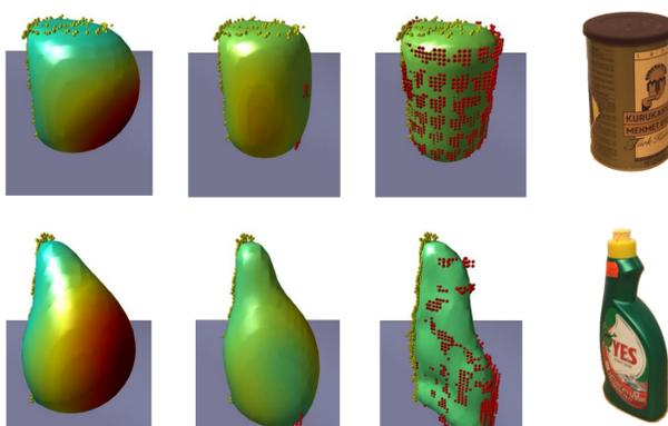
Evolution of implicit shape approximation as more tactile data becomes available and where the objects are positioned to show the back-side not visible from a single-view kinect capture (from [1]).
