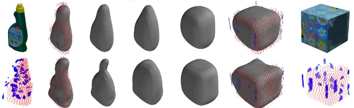
Shape approximations from haptic (blue) and single-view kinect (red) data and shape deformations using a convex combination of the corresponding GP means.
