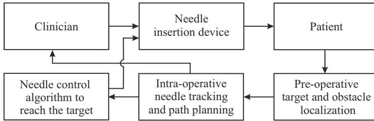
**Fig. 2** The workflow presents a clinically viable robotic needle steering system. The needle insertion device controls the direction of insertion inside the patient’s soft tissue. Needle tip tracking and path planning are performed intra-operatively to provide control algorithm and the clinician with data required to control the insertion device.
