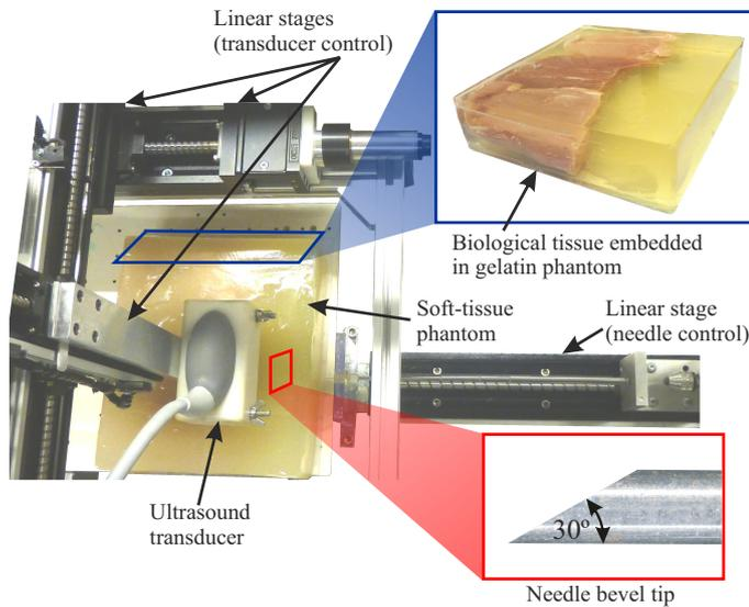
**Fig. 1** The experimental setup shows the needle insertion device and the transducer control device. The upper inset depicts biological tissue (chicken breast) embedded in a gelatin phantom. The lower inset shows the needle bevel tip.
