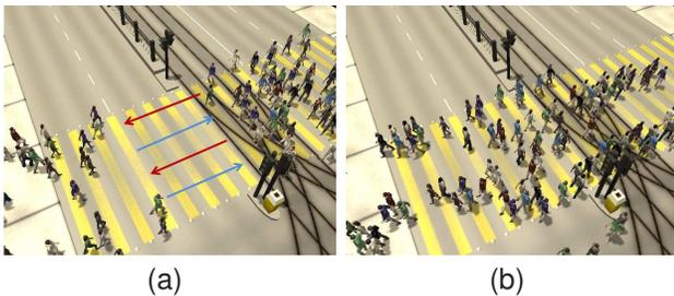
**Fig. 4: Crosswalk Simulation:** (a) Sketch-based guidance fields to specify lane formation in the simulation; (b) Lane formation generated by goal-directed navigation fields.
