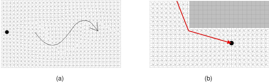
**Fig. 8: Navigation fields** (a) A navigation field computed for the guidance field shown in Figure 3 (and indicated by the arrow here) with the goal (black dot) placed such that the guidance field points away from it. (b) If there is no guidance field, the navigation field gives the shortest paths to the goal (black dot). A shortest path is shown with a sharp turn at the obstacle (light gray) corner.
