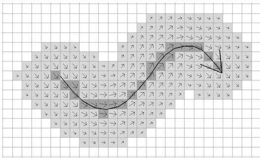
**Fig. 3: Sketching interface for specifying gradients** A user drawn stroke is rasterized onto the regular grid and a region of influence of user-specified width is constructed around the skeleton of the stroke. The gradients along the sketched curve are propagated to grid cells within this region.
