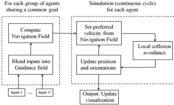
**Fig. 2: A schematic overview of our method** For every distinct group of agents sharing a common objective, a goal-directed navigation field is interactively computed. This is used to drive individual agents at every simulation time-step. The agents run a continuous cycle of sensing and acting (as depicted by the right-hand box).
