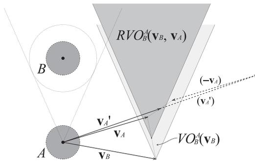
**Fig. 11: The Reciprocal Velocity Obstacle  $RVO_B^A(\mathbf{v}_B, \mathbf{v}_A)$  of agent B to agent A. It is used for local collision avoidance. We compute this locally for each agent during each simulation cycle.**
