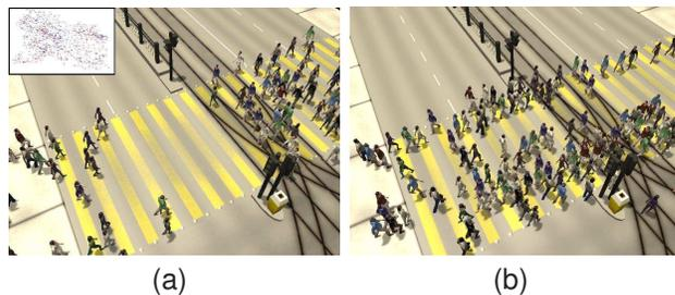
**Fig. 6: Crosswalk Simulation:** (a) Video-based motion patterns from Figure 5(e) used as guidance fields; (b) Agent motion generated by the navigation fields.
